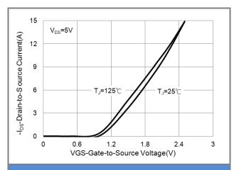
**Fig.2 Transfer Characteristics**
