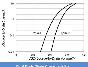
Fig.6 Body Diode Characteristics
