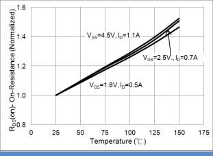
Fig.4 On-Resistance vs. Junction temperature
