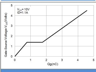
Fig.7 Gate-Charge Characteristics
