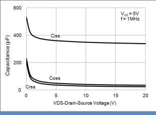
Fig.9 Capacitance vs. Drain-Source Voltage
