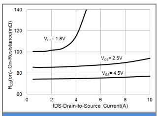
Fig.3 On-Resistance vs. Drain Current
