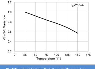
Fig.8 Threshold Voltage Variation with Temperature
