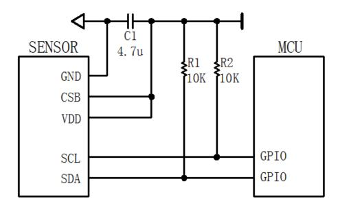
Figure2: Typical application circuit
