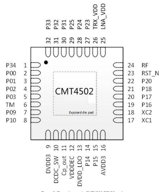
Figure 2: Pin assignment - CMT4502 QFN32 package
