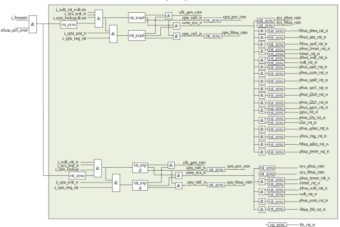
Figure 6: CMT4502 power, clock and reset
