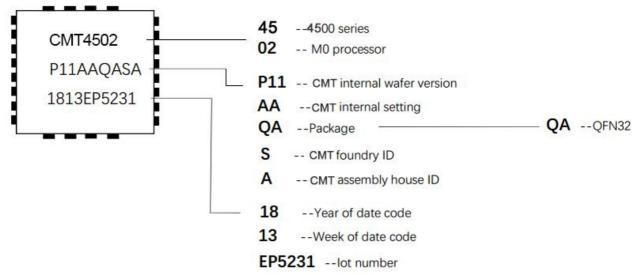
Figure 14: Chip Marking
