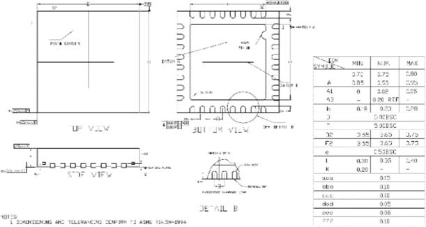
Figure 15: QFN32 package dimensions
