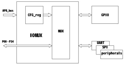
Figure 10: IOMUX structure diagram
