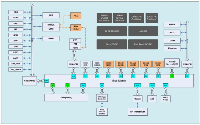
Figure 1: CMT4502 block diagram
