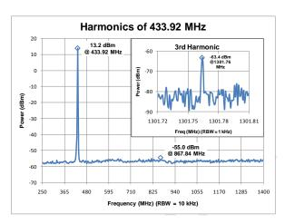
Figure 5. Harmonics of 433.92 MHz,  $P_{OUT} = +13 \text{ dBm}$
