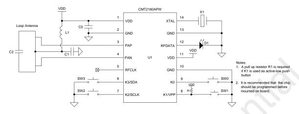
Figure 1. CMT2180APW Typical Application with Differential PA Output
