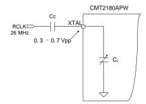
Figure 16. XTAL Circuitry and Crystal Model
