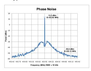
Figure 4. Phase Noise,  $F_{RF} = 433.92$  MHz,  $P_{OUT} = +13$  dBm, Unmodulated
