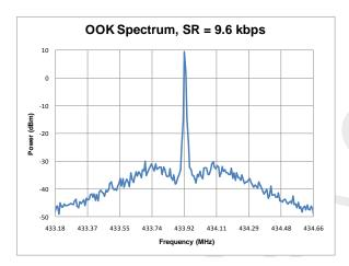
Figure 7. OOK Spectrum, SR = 9.6 ksps,  $P_{OUT}$  = +10 dBm,  $t_{RAMP}$  = 32 us
