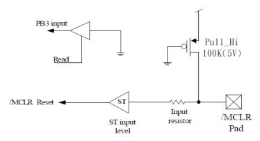
Figure 32. /MCLR Equivalent Circuit
