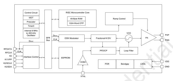
Figure 12. CMT2180APW Functional Block Diagram
