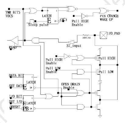
Figure 33. PB4 Equivalent Circuit
