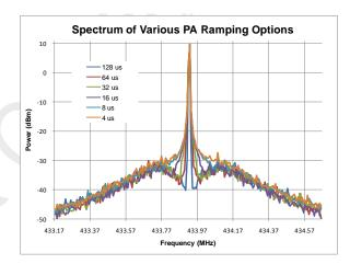
Figure 6. Spectrum of PA Ramping,  $SR = 9.6 \text{ ksps}, P_{OUT} = +10 \text{ dBm}$
