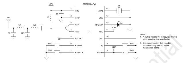
Figure 11. CMT2180APW Typical Application with Single-ended PA Output
