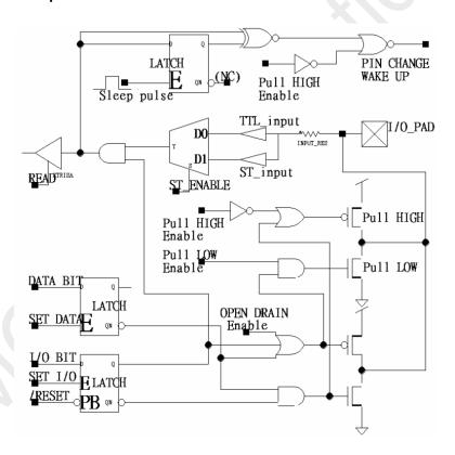
Figure 29. PB0 ,PB1 ,PB5 Equivalent Circuit
