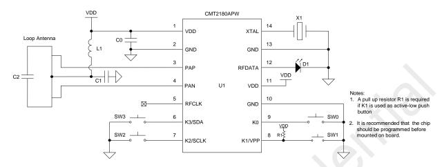
Figure 10. CMT2180APW Typical Application with Differential PA Output
