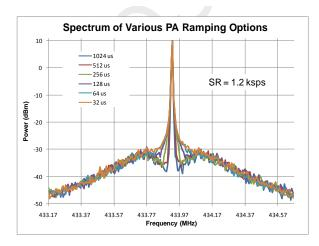
Figure 8. Spectrum of PA Ramping, SR = 1.2 ksps, P<sub>OUT</sub> = +10 dBm
