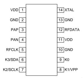
Figure 3. CMT2180APW Pin Assignments
