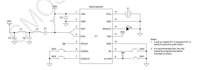
Figure 2. CMT2180APW Typical Application with Single-ended PA Output
