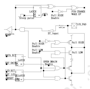
Figure 30. PB2 Equivalent Circuit
