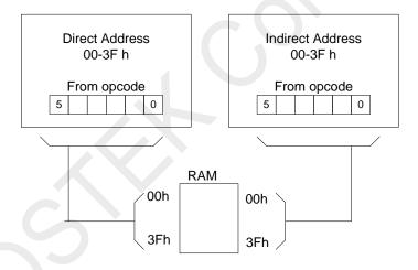
Figure 27. Direct/Indirect Addressing
