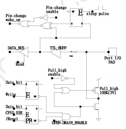
Figure 31. PB3 Equivalent Circuit
