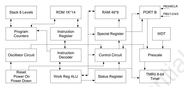
Figure 23. Microcontroller Core Block Diagram
