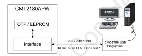
Figure 13. Accessing Embedded OTP / EEPROM
