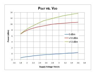
Figure 9. Output Power vs. Supply Voltages, F<sub>RF</sub> = 433.92 MHz
