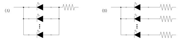
• This product should be operated in forward bias. A driving circuit must be designed so that the product is not subjected to either forward or reverse voltage while it is off. In particular, if a reverse voltage is continuously applied to the product; such operation can cause migration resulting in LED damage.
