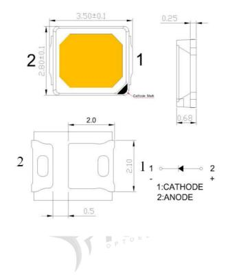
Recommend Soldering pad design(unit=mm)
