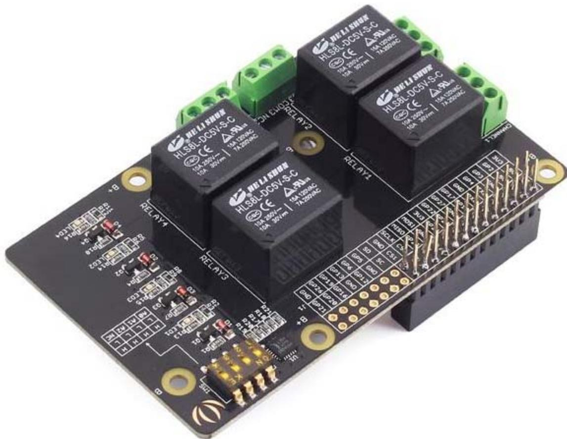
The Relay Shield utilizes four high quality relays and provides NO/NC interfaces that control the load of high current. Which means it could be a nice solution for controlling devices that couldn't be directly controlled by IIC bus. Standardized shield form factor enables smoothly connection with the Raspberry Pi. The shield also has four dynamic indicators show the on/off state of each relay.
