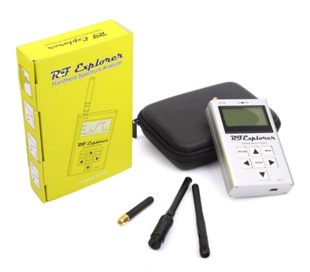
RF Explorer 6G Combo is a handheld digital spectrum analyzer, a very affordable tool for work in all popular frequency bands. It is based on a highly integrated frequency synthesizer and double balanced mixer which offers high performance, compact size, low consumption and low cost.
