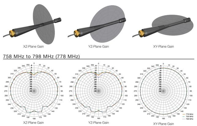
Figure 9. Radiation Patterns for PW LTE Band 14 Antenna
