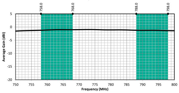
Figure 5. PW LTE Band 14 Antenna Average Gain with Band 14 Uplink/Downlink Highlights
