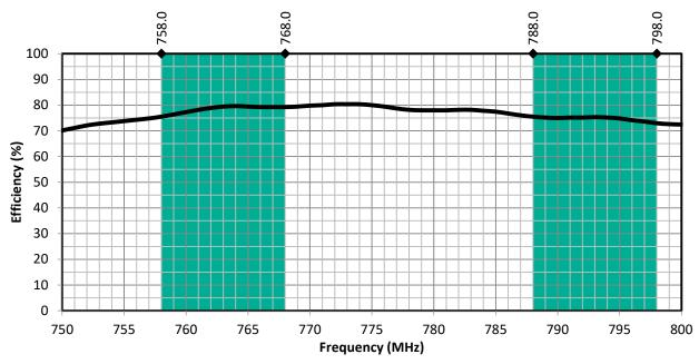
Figure 6. PW LTE Band 14 Antenna Radiation Efficiency with Band 14 Uplink/Downlink Highlights
