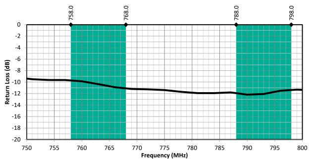
Figure 3. PW LTE Band 14 Antenna Return Loss with Band 14 Uplink/Downlink Highlights
