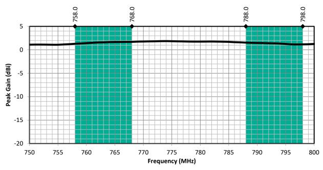
Figure 4. PW LTE Band 14 Antenna Peak Gain with Band 14 Uplink/Downlink Highlights
