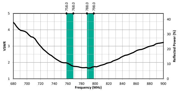
Figure 2. PW LTE Band 14 Antenna Full Bandwidth VSWR
