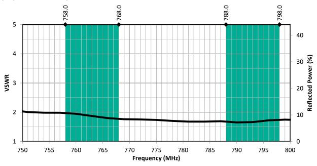
Figure 1. PW LTE Band 14 Antenna VSWR with Band 14 Uplink/Downlink Highlights
