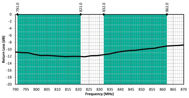
Figure 3. PW LTE Band 20 Antenna Return Loss with Band 20 Uplink/Downlink Highlights
