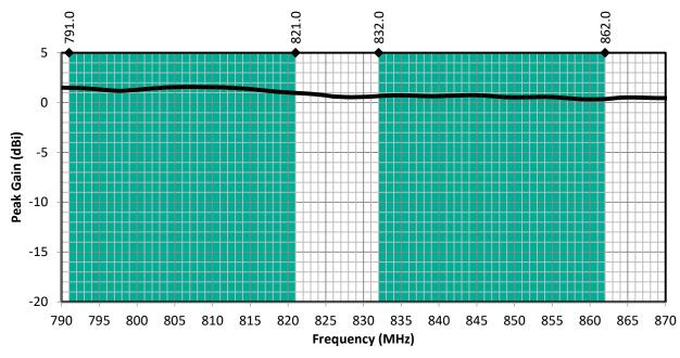
Figure 4. PW LTE Band 20 Antenna Peak Gain with Band 20 Uplink/Downlink Highlights
