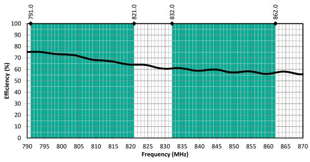
Figure 6. PW LTE Band 20 Antenna Radiation Efficiency with Band 20 Uplink/Downlink Highlights
