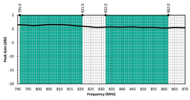
Figure 4. CW LTE Band 20 Antenna Peak Gain with Band 20 Uplink/Downlink Highlights
