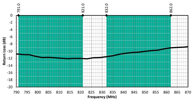
Figure 3. CW LTE Band 20 Antenna Return Loss with Band 20 Uplink/Downlink Highlights
