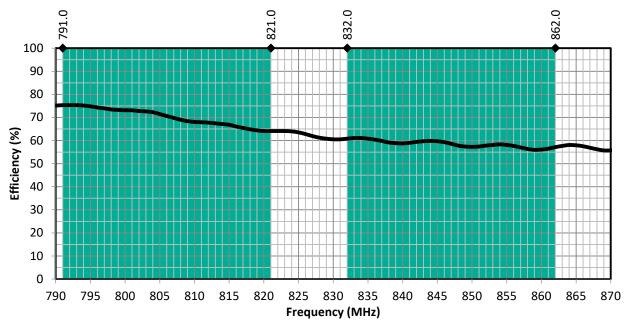
Figure 6. CW LTE Band 20 Antenna Radiation Efficiency with Band 20 Uplink/Downlink Highlights
