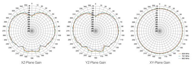
Figure 9. Radiation Patterns for CW LTE Band 20 Antenna
