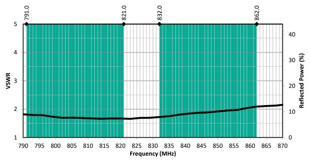
Figure 1. CW LTE Band 20 Antenna VSWR with Band 20 Uplink/Downlink Highlights
