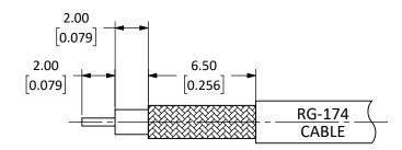
RECOMMENDED CABLE STRIPPING DIMENSIONS CAN ALSO BE USED WITH: RG-188A & RG-316
