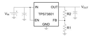
Figure 24. Adjustable Operation
