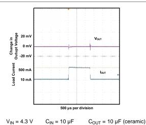
Figure 21. Load Transient Response
