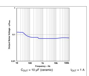
Figure 20. Output Noise Voltage vs Frequency
