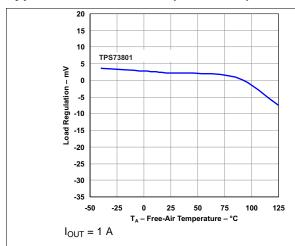
Figure 19. Load Regulation vs Temperature
