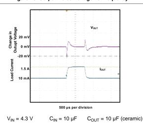
Figure 22. Load Transient Response
