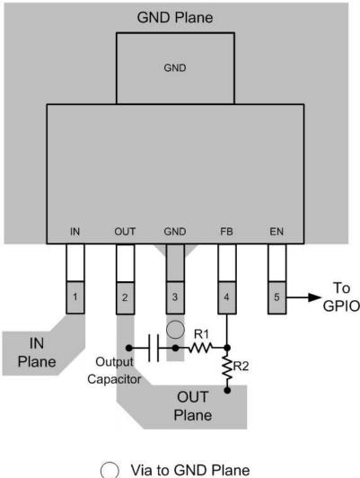
Figure 28. SOT-223 Layout Example (DCQ)
