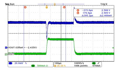
Figure 27. 1-A Load Transient Response
