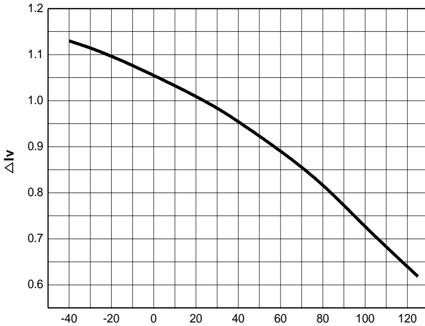
Fig 6. Relative Light Output vs. Junction Temperature, I_F = 20\text{mA}
