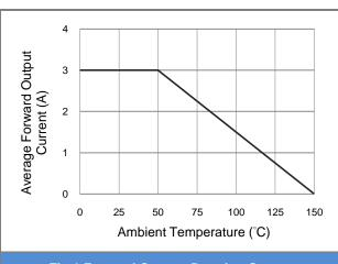
Fig.1 Forward Current Derating Curve
