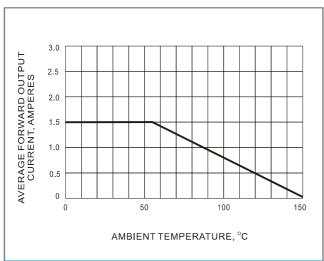
FIG.1 DERATING CURVE FOR OUTPUT RECTIFIED CURRENT
