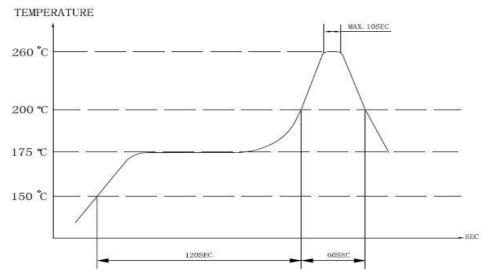
Heat resistant line Used when heat resistant reliability test is performed
