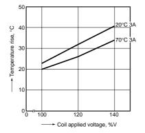
3. Ambient temperature characteristics and coil applied voltage
