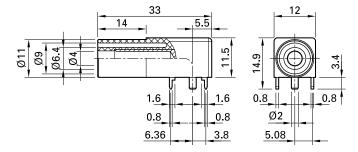
Insulated, right-angled Ø 4 mm rigid socket accepting springloaded Ø 4 mm plugs with rigid insulating sleeve. Machined brass.Connection: Ø 2 mm round pin and contacts for mounting on printed circuit boards.
