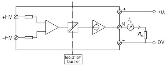
Figure 14: standard characterization schematics for current output transducers ( $R_M = 50 \Omega$  unless otherwise noted)
