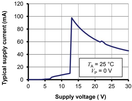
Figure 6: Supply current function of supply voltage
