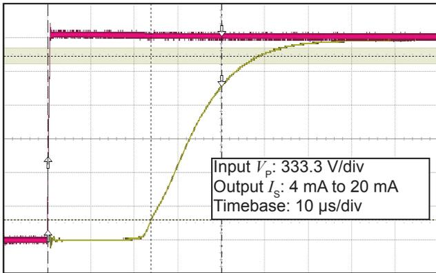
Figure 10: Typical step response (0 to  $V_{PN}$ )
