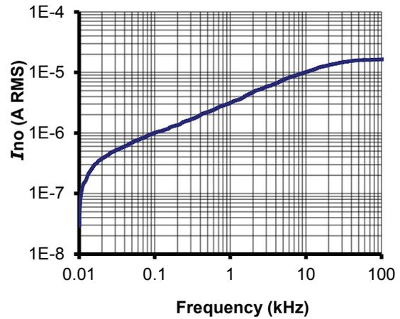
Figure 13: Typical total output RMS noise current with  $R_M = 50 \Omega$
