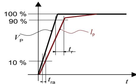
Figure 15: response time  $t_r$  and reaction time  $t_{ra}$
