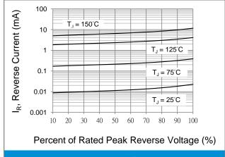
Fig.3 Typical Reverse Characteristics
