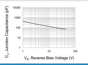
Fig.2 Typical Junction Capacitance
