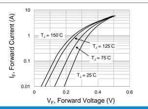
Fig.4 Typical Forward Characteristics
