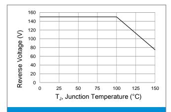
**Fig.5 Operating Temperature Derating Curve**
