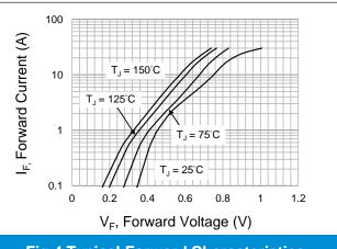
**Fig.4 Typical Forward Characteristics**
