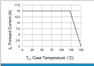
**Fig.1 Forward Current Derating Curve**
