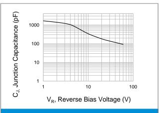
Fig.2 Typical Junction Capacitance
