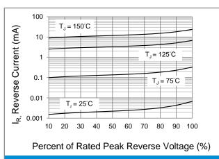
Fig.3 Typical Reverse Characteristics
