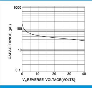
FIG.3-TYPICAL JUNCTION CHATACTERISTIC
