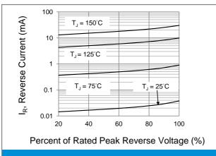
Fig.3 Typical Reverse Characteristics
