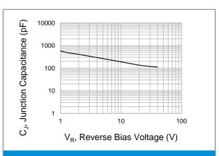
**Fig.2 Typical Junction Capacitance**
