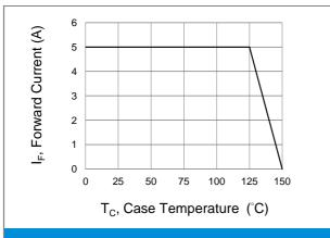
**Fig.1 Forward Current Derating Curve**
