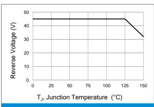
**Fig.5 Operating Temperature Derating Curve**
