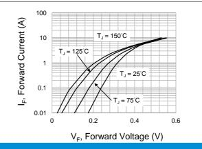
**Fig.4 Typical Forward Characteristics**
