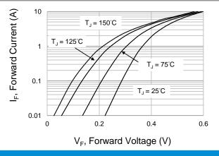
Fig.4 Typical Forward Characteristics
