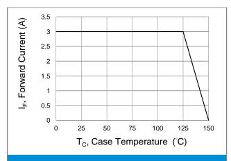
**Fig.1 Forward Current Derating Curve**
