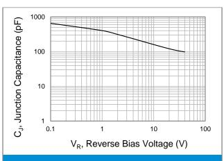
Fig.2 Typical Junction Capacitance
