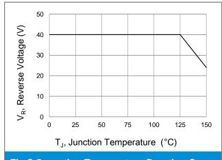
**Fig.5 Operating Temperature Derating Curve**
