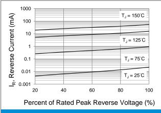
Fig.3 Typical Reverse Characteristics
