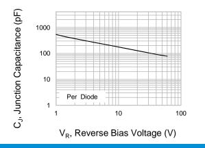
Fig.2 Typical Junction Capacitance
