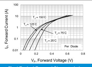
Fig.4 Typical Forward Characteristics
