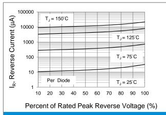
**Fig.3 Typical Reverse Characteristics**
