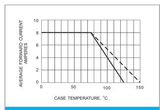
Fig.1- FORWARD CURRENT DERATING CURVE
