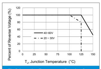
**Fig.5 Operating Temperature Derating Curve**
