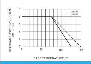
Fig. 1-FORWARD CURRENT DERATING CURVE
