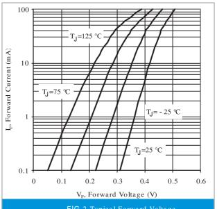
FIG.2-Typical Forward Voltage
