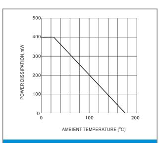
Fig.2 POWER DISSIPATION DERATING CURVE
