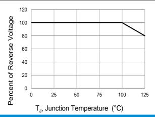
**Fig.4 Operating Temperature Derating Curve**
