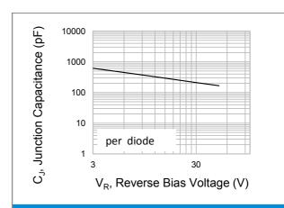
**Fig.2 Typical Junction Capacitance**
