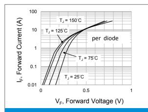
**Fig.4 Typical Forward Characteristics**
