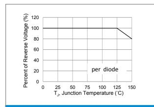
**Fig.5 Operating Temperature Derating Curve**
