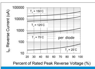
Fig.3 Typical Reverse Characteristics
