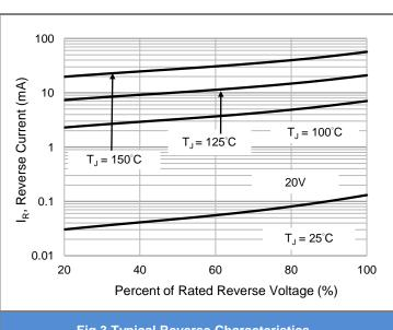
Fig.3 Typical Reverse Characteristics
