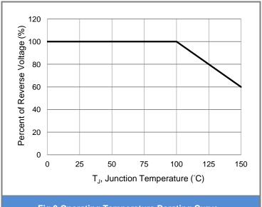
**Fig.9 Operating Temperature Derating Curve**
