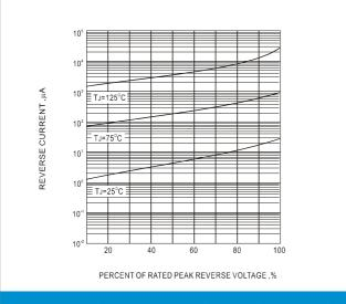
Fig.3 TYPICAL REVERSE CHARACTERISTIC
