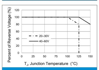
**Fig.5 Operating Temperature Derating Curve**
