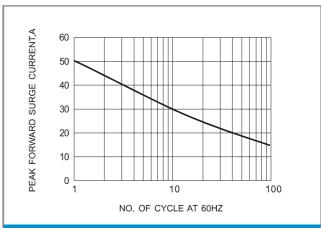
Fig.2 MAXIMUM NON-REPETITIVEPEAKFORWARD SURGE CURRENT
