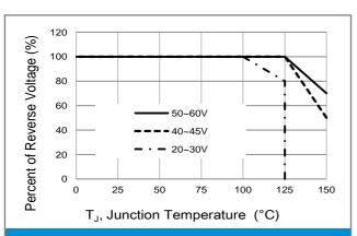
**Fig.5 Operating Temperature Derating Curve**
