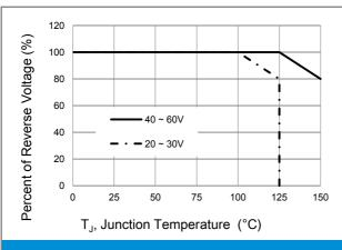
**Fig.5 Operating Temperature Derating Curve**
