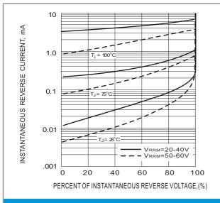
Fig.3 TYPICAL REVERSE CHARACTERISTIC
