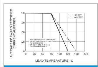
Fig.1 FORWARD CURRENT DERATING CURVE
