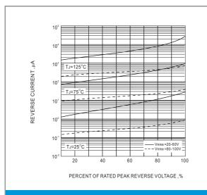
Fig.3 TYPICAL REVERSE CHARACTERISTIC
