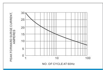
Fig.2 MAXIMUM NON-REPETITIVEPEAKFORWARD SURGE CURRENT
