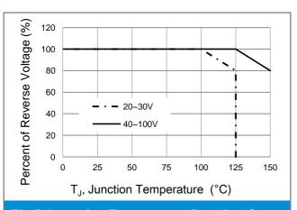
**Fig.5 Operating Temperature Derating Curve**
