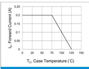
Fig.1 Forward Current Derating Curve
