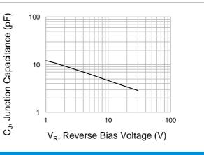
Fig.2 Typical Junction Capacitance
