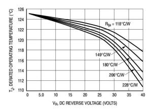
Fig. 3. Typical Operating Temperature Derating
