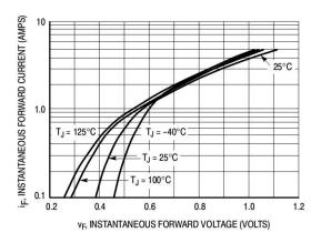
Fig. 1. Typical Forward Voltage
