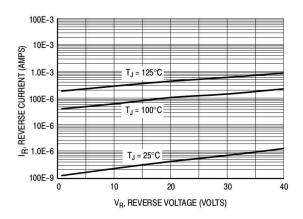
Fig. 2. Typical Reverse Current
