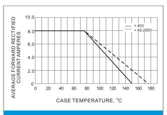
Fig.1- FORWARD CURRENT DERATING CURVE
