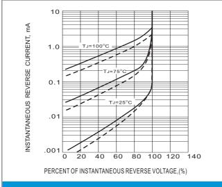
Fig.3- TYPICAL REVERSE CHARACTERISTICS
