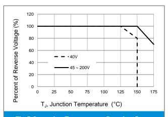
**Fig.5 Operating Temperature Derating Curve**
