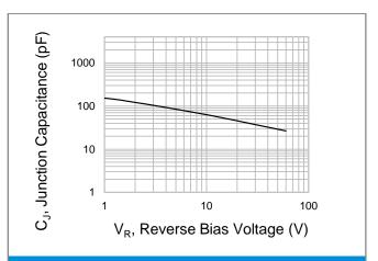
**Fig.2 Typical Junction Capacitance**
