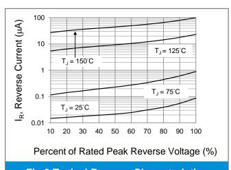
**Fig.3 Typical Reverse Characteristics**
