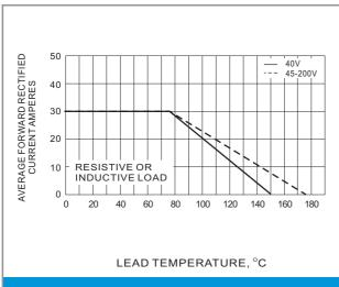
Fig.1 FORWARD CURRENT DERATING CURVE
