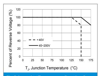
Fig.5 Operating Temperature Derating Curve
