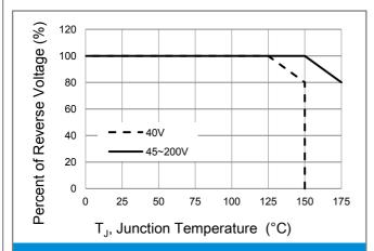
Fig.5 Operating Temperature Derating Curve
