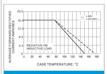
Fig.1 FORWARD CURRENT DERATING CURVE
