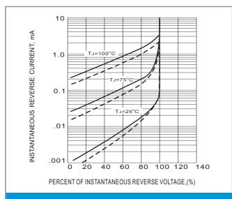
Fig.3 TYPICAL REVERSE CHARACTERISTICS
