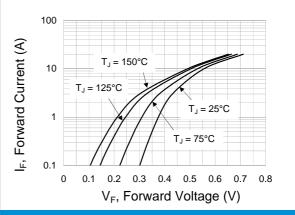
**Fig.4 Typical Forward Characteristics**
