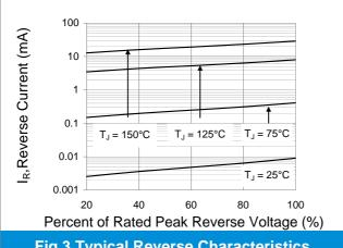
Fig.3 Typical Reverse Characteristics
