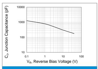
**Fig.2 Typical Junction Capacitance**
