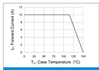
**Fig.1 Forward Current Derating Curve**
