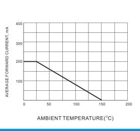
FIG. 4 FORWARD CURRENT DERATING
