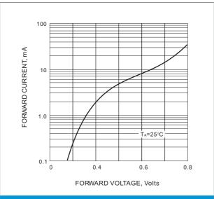
FIG. 1 TYPICAL FORWARD CHARACTERISTIC
