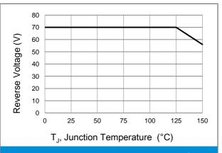
**Fig.5 Operating Temperature Derating Curve**
