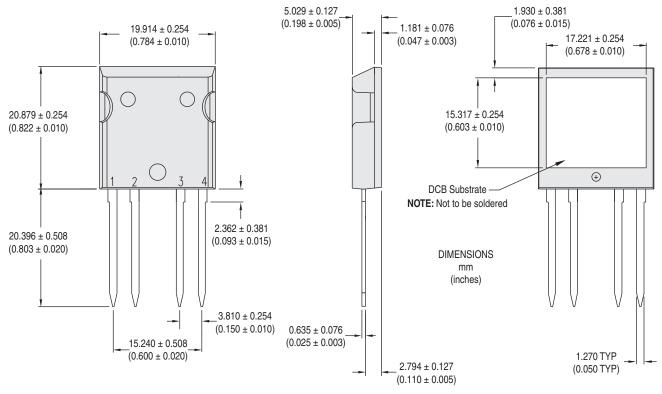
**NOTE:** Metallized external surface of DCB substrate maintains 2500V<sub>rms</sub> isolation to device internal structure and all external pins.
