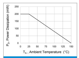
**Fig.1 Power Derating Curve**
