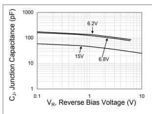
Fig.2 Typical Junction Capacitance
