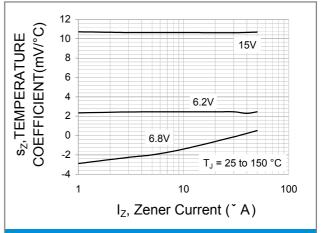
Fig.6 Temperature coefficient as a function of working current; typical values
