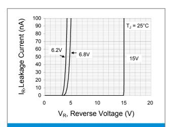
Fig.3 Typical Leakage Characteristics
