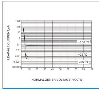
Fig.2 TYPICAL LEAKAGE CURRENT
