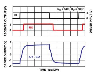
FIGURE 27.  $V_{CC}$  = 3.3V, DRIVER AND RECEIVER WAVEFORMS (ISL32450E, ISL32452E, ISL32457E)
