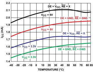
FIGURE 14. SUPPLY CURRENT vs TEMPERATURE
