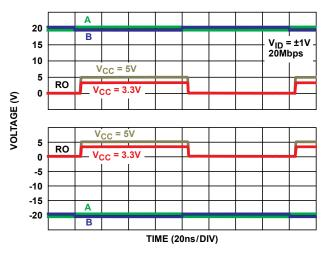
FIGURE 26. ±20V RECEIVER PERFORMANCE (ISL32458E, ISL32459E)
