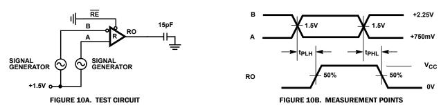
FIGURE 10. RECEIVER PROPAGATION DELAY AND DATA RATE
