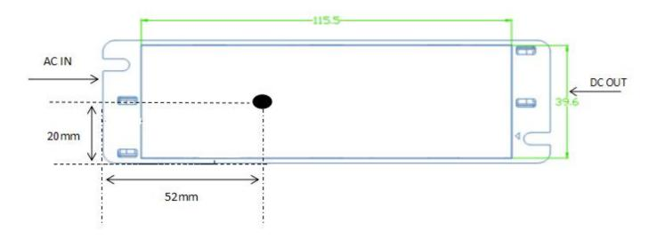
4. Dimensional Drawing (unit: mm, tolerance:  $\pm 0.5$ mm)
