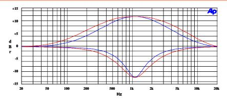
Figure 29: EQ Band 3, EQ3BW = 0 versus EQ3BW = 1
