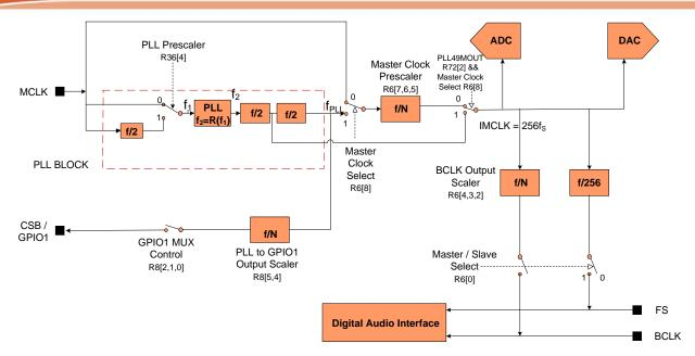
Figure 14: PLL and Clock Select Circuit
