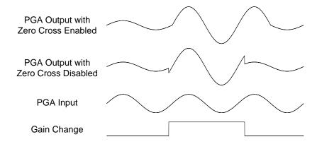
Figure 2: Zero Crossing Gain Update Operation
