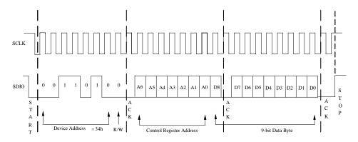
Figure 20: Byte Write Sequence
