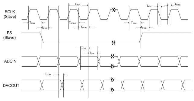
Figure 34: Digital Audio Interface Slave Mode Timing
