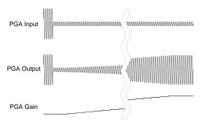
Figure 9: ALC Operation Without Noise Gate
