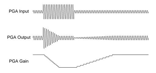
Figure 7: ALC Normal Mode Operation
