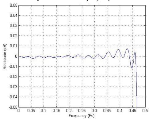
Figure 20: ADC Filter Ripple
