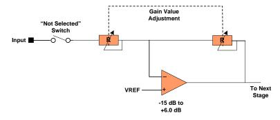
Figure 5: Variable Gain Stage Simplified Schematic
