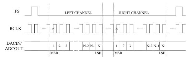
Figure 30: PCM Time Slot Audio Interface
