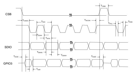
Figure 32: 4-wire Control Mode Timing
