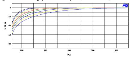
Figure 23: ADC Highpass Filter Response, HPF enabled, FS = 24kHz
