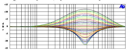
Figure 30: EQ Band 4 Peak Filter Gains for Lowest Cut-Off Frequencies with EQ4BW = 0
