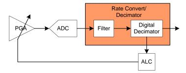
Figure 6: ALC Block Diagram
