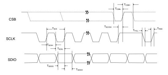
Figure 31: 3-wire Control Mode Timing
