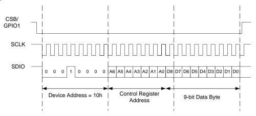
Figure 23: Register Write operation using a 24-bit SPI Interface
