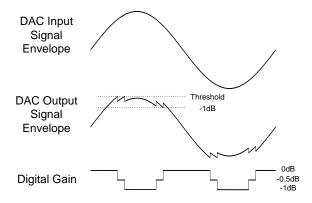
Figure 13: DAC Digital Limiter Control
