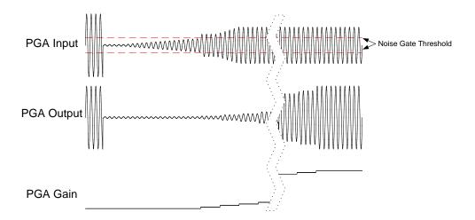
Figure 10: Noise Gate Operation
