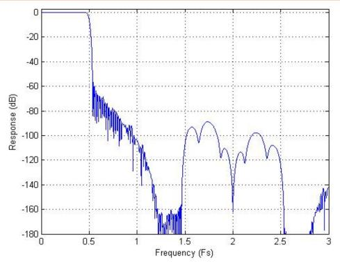
Figure 19: ADC Filter Frequency Response
