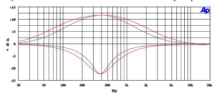
Figure 27: EQ Band 2, EQ2BW = 0 versus EQ2BW = 1
