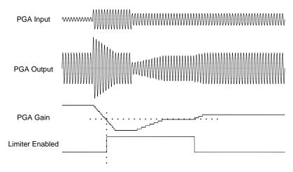
Figure 12: ALC Limiter Mode Operation
