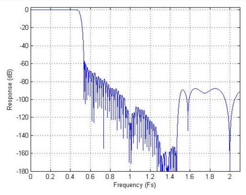
Figure 17: DAC Filter Frequency Response
