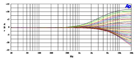
Figure 32: EQ Band 5 Gains for Lowest Cut-Off Frequency
