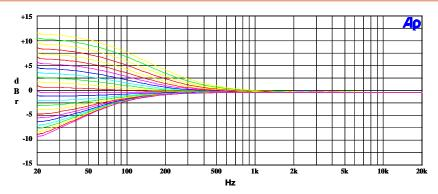
Figure 25: EQ Band 1 Gains for Lowest Cut-Off Frequency
