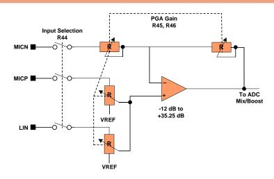
Figure 3: PGA Input Structure Simplified Schematic
