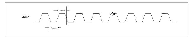
Figure 15: MCLK Timing Diagram
