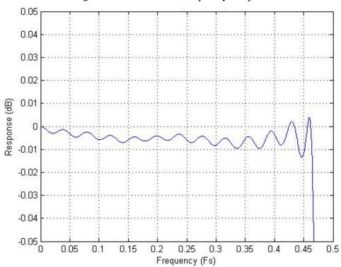
Figure 18: DAC Filter Ripple
