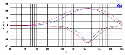
Figure 31: EQ Band 4, EQ4BW = 0 versus EQ4BW =1
