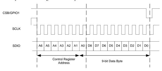
Figure 22: Register write operation using a 16-bit SPI Interface
