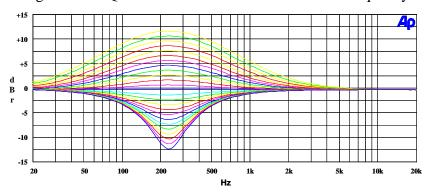
Figure 26: EQ Band 2 Peak Filter Gains for Lowest Cut-Off Frequency with EQ2BW = 0
