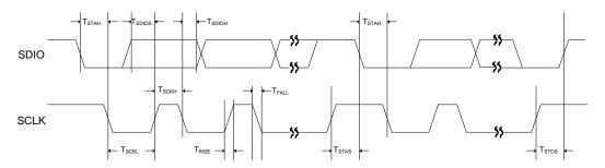
Figure 33: Two-wire Control Mode Timing
